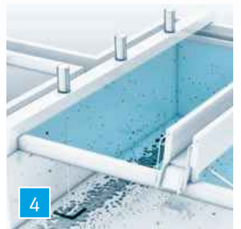
4 Sedimentation tank Controlling sludge discharge using poppet valves
